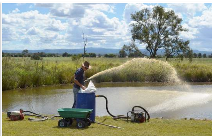
Figure 7. Treatment to a smaller waterbody using a land-based application system
