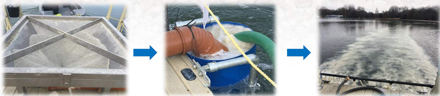
Figure 4. Diagram of the Phoslock application process, with Phoslock in its granule form (left), granules being mixed with lake water (middle) and then applied to the surface of a waterbody (right)
